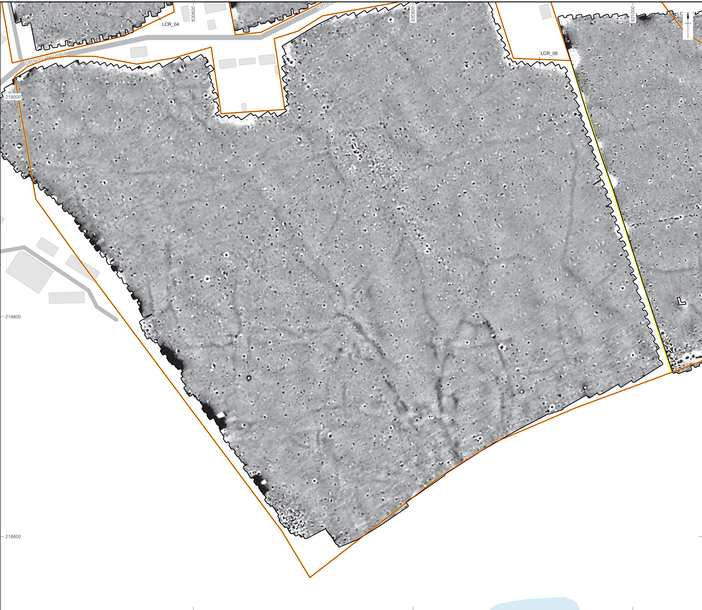
Figure 108: Gradiometer survey results: greyscale plot (LCR_07, LCR_06, LCR_04)
