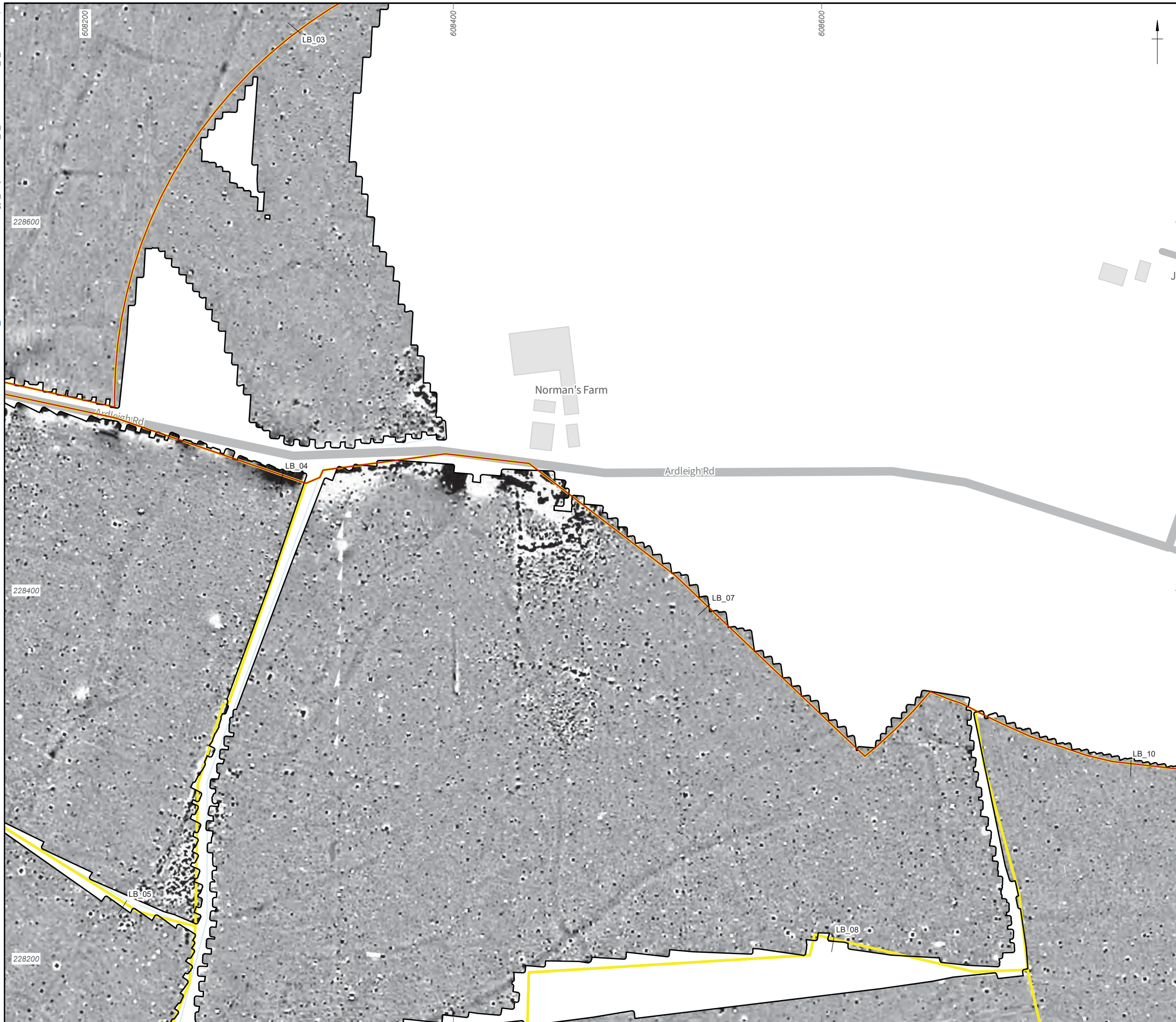
Figure 20: Gradiometer survey results: greyscale plot (LB_03, LB_07, LB_04, LB_05, LB_08, LB_10)
