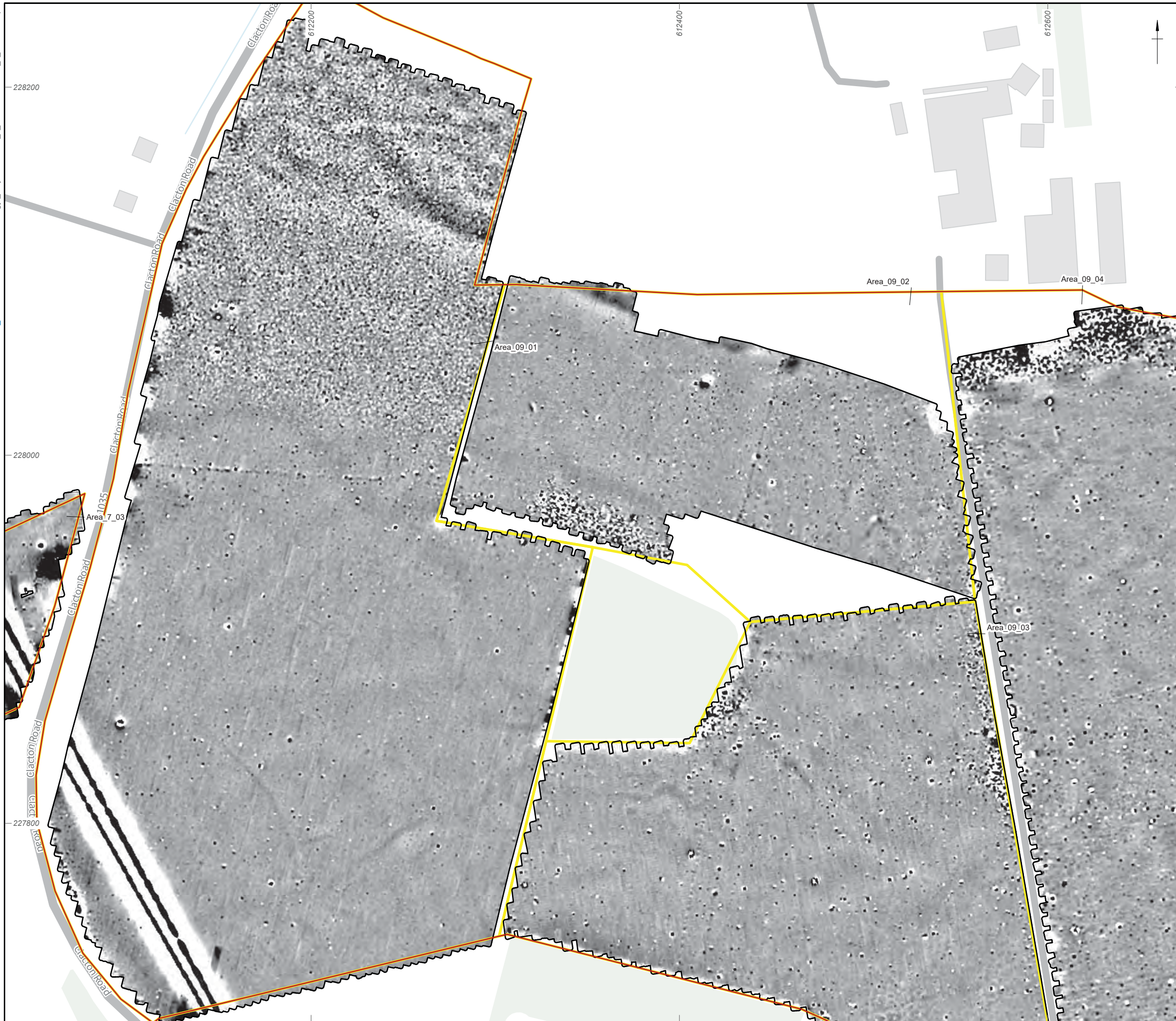
Figure 46: Gradiometer survey results: greyscale plot (Area_09_04, Area_09_03, Area_09_02, Area_09_01, Area_7_03)
